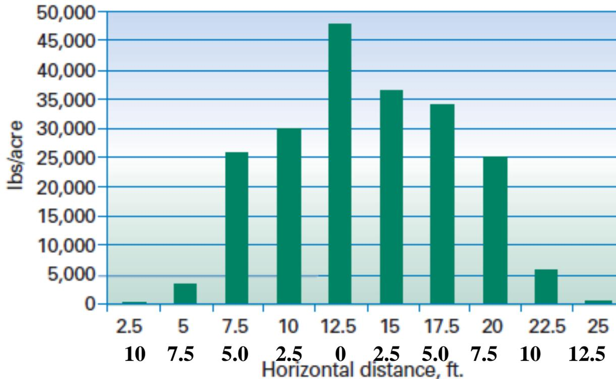
Figure 2. Typical single-swath pattern for a rear-beater spreader.
