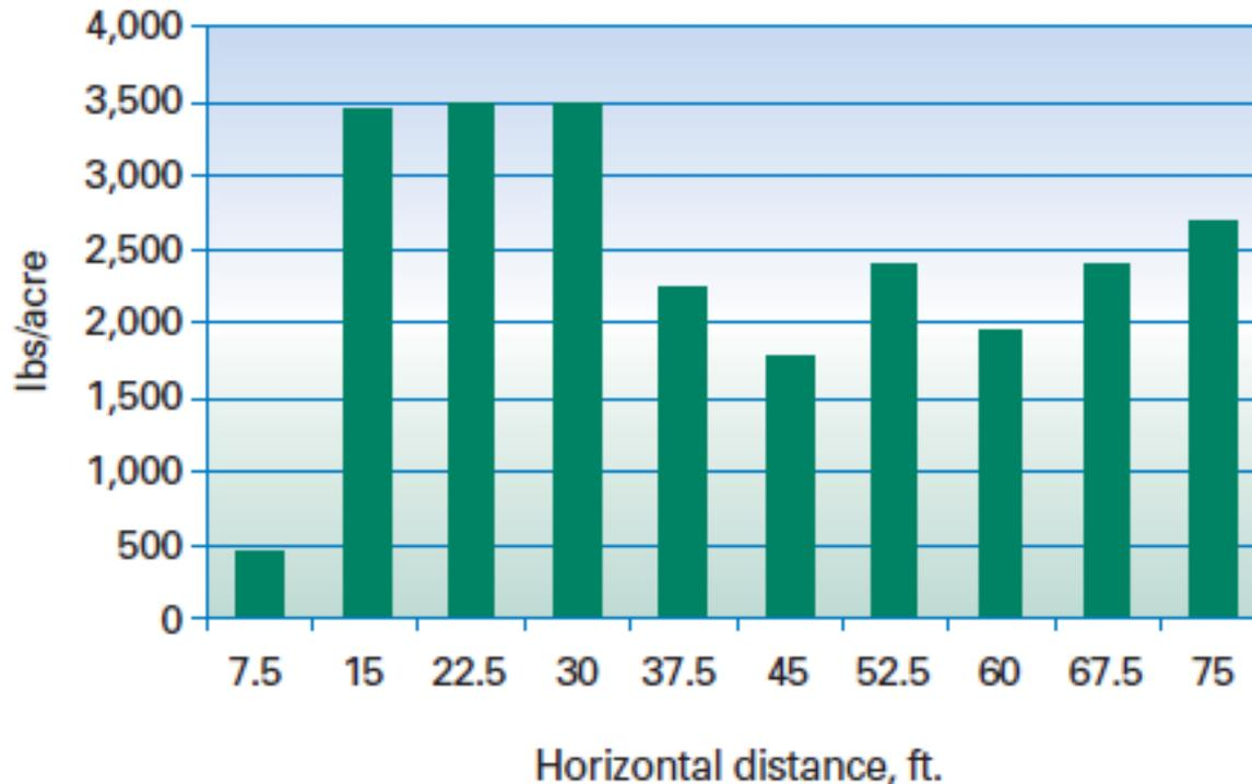
Figure 6. Typical single-swath pattern for side-delivery spreader.
